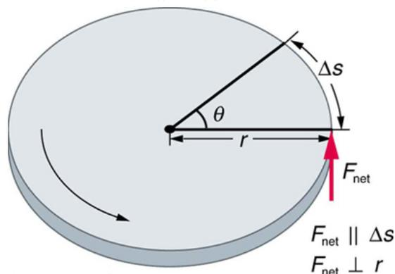
**Figure 10.15** The net force on this disk is kept perpendicular to its radius as the force causes the disk to rotate. The net work done is thus  $(\text{net } F)\Delta s$ . The net work goes into rotational kinetic energy.
