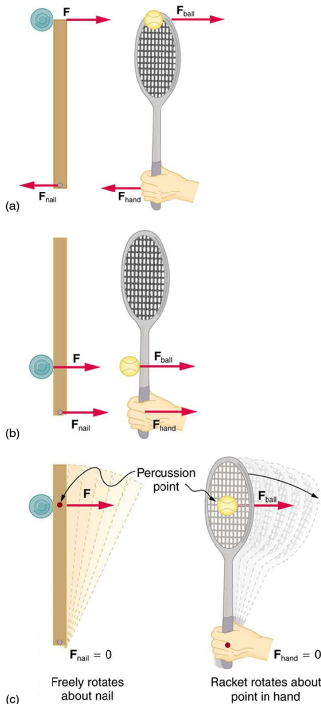
**Figure 10.27** A disk hitting a stick is compared to a tennis ball being hit by a racquet. (a) When the ball strikes the racquet near the end, a backward force is exerted on the hand. (b) When the racquet is struck much farther down, a forward force is exerted on the hand. (c) When the racquet is struck at the percussion point, no force is delivered to the hand.
