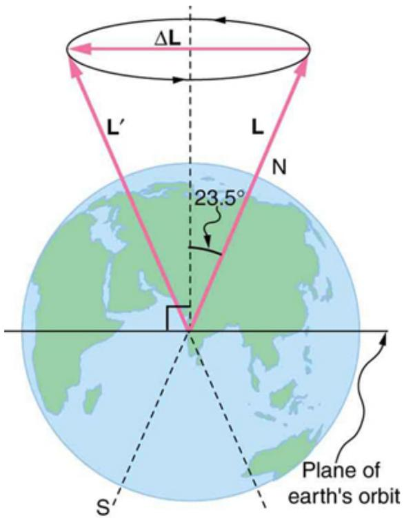
**Figure 10.41** The Earth's axis slowly precesses, always making an angle of  $23.5^\circ$  with the direction perpendicular to the plane of Earth's orbit. The change in angular momentum for the two shown positions is quite large, although the magnitude  $L$  is unchanged.
