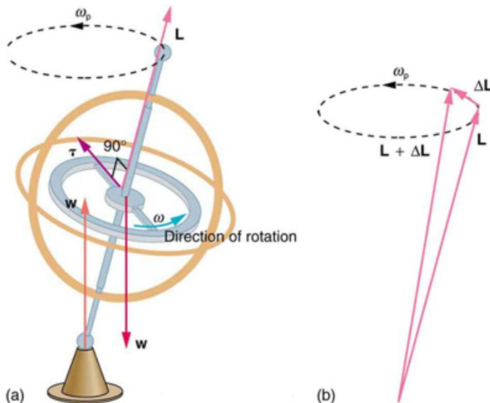
**Figure 10.31** As seen in figure (a), the forces on a spinning gyroscope are its weight and the supporting force from the stand. These forces create a horizontal torque on the gyroscope, which create a change in angular momentum  $\Delta\mathbf{L}$  that is also horizontal. In figure (b),  $\Delta\mathbf{L}$  and  $\mathbf{L}$  add to produce a new angular momentum with the same magnitude, but different direction, so that the gyroscope precesses in the direction shown instead of falling over.
