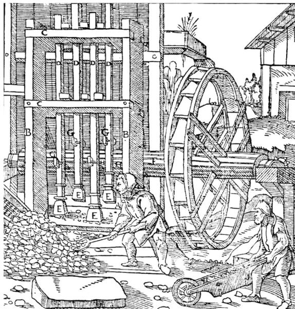
**Figure 9.36:** The cam principle as applied to a rock-crushing mill illustrated by Georgius Agricola in his book *De Re Metallica* (1556).
